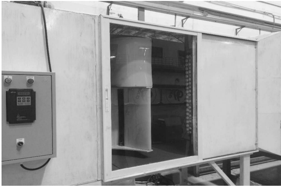
Figure 4 An experimental wind tunnel measuring a vertical wind turbine
